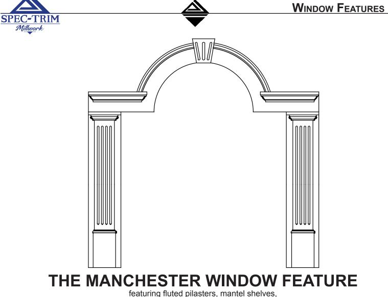
flat casing with rakemoulding and a fluted key.
